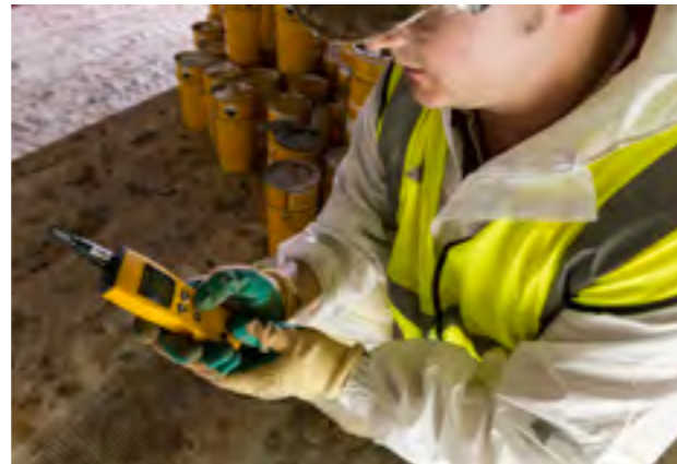
Measuring the ambient temperature and relative humidity.
