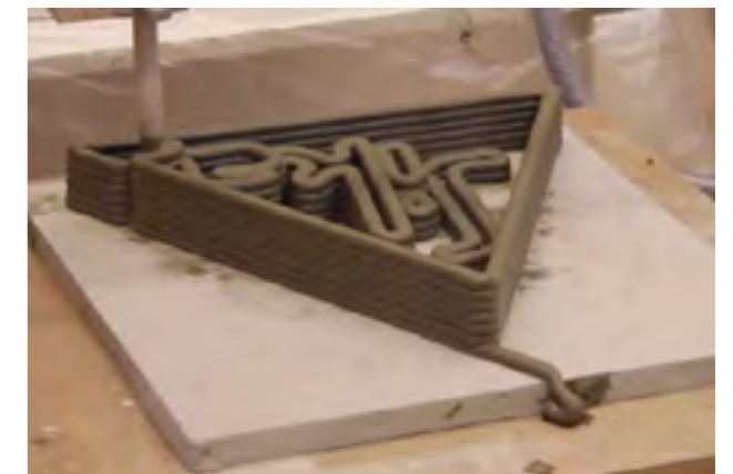
Figure 2: Combination of a robotic arm with the MiniShot system; 3D Sika logo
