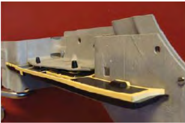
SikaBaffle® -450 in JLR X760 cavity left before and right after baking.
