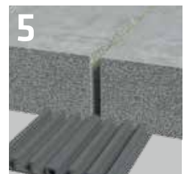
Expansion joints under base plates
