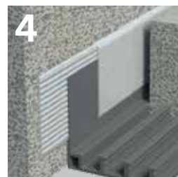
Connection joints to existing components
