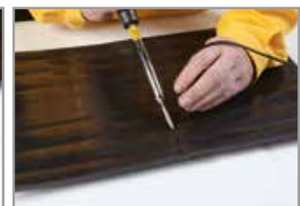
Strengthening with welding strip using welding tip
