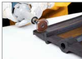
Grinding of the rubber surface
