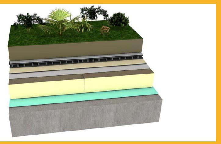
SIKAPLAN® PVC - GREEN ROOF SYSTEM - INTENSIVE ON CONCRETE DECK WITH THERMAL INSULATION TECHNICAL DETAILS SPL PVC - 051.
