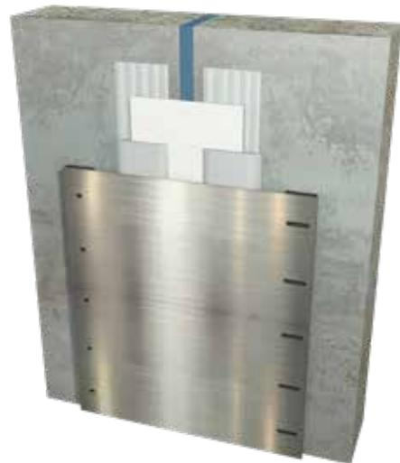
E.g. external basement walls. For exposure to negative water pressure from outside, the Sikadur Combiflex® SG Tape must be secured with a steel plate fixed on one side of the joint.
