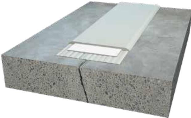
**Construction joints** are formed by the operational subdivision of structures into sections, such as for the daily completion of concreting stages (also called "day work joints").
