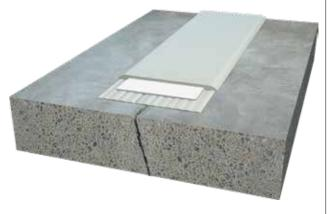
**Construction joints** are formed by the operational subdivision of structures into sections, such as for the daily completion of concreting stages (also called "day work joints").
