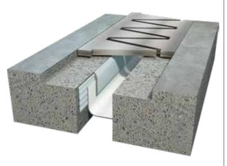
Typical for use on bridge deck joints or on multi-storey car park deck joints.
