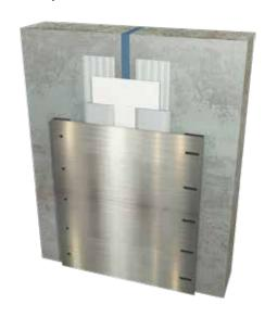
E.g. external basement walls. For exposure to negative water pressure from outside, the Sikadur Combiflex® SG Tape must be secured with a steel plate fixed on one side of the joint.
