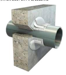
Basement wall with power and water services entry ducts.
