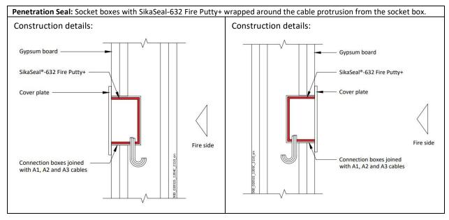
A.1.2.1 Single side penetration seal with cables in socket boxes
