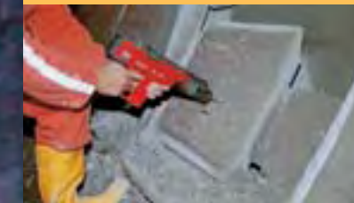
Early strength of 1 – 15 N/mm² Stud-shooting method 4
