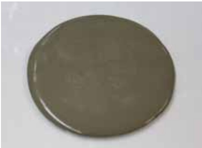
Cement mortar paste includes all binders, powder additives and the free water (not absorbed by the aggregates). Fine mortar paste includes in addition also all fine parts of the aggregates \leq 0.125 mm.
