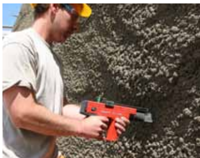
Fig. 8-13/14: Penetration of young sprayed concrete with studs using a Hilti DX 450-SCT (left) and measurement of the stud standoff for the determination of the penetration
