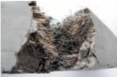
Fig. 5-2: Well distributed fibers in concrete
