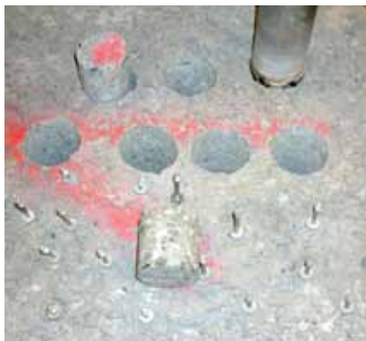
Fig. 8-15 / 16: Core drilling from sprayed concrete sample (left) and compressive strength measurement of a drill core (right)
