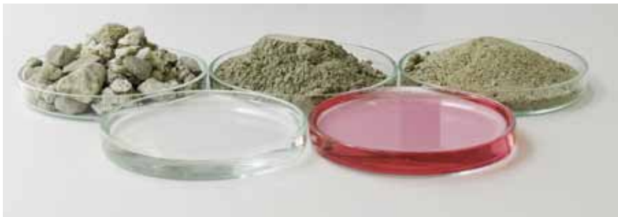
Fig. 6-1: Mix design ingredients of shotcrete: Gravel, water, cement, superplasticizer, sand (from left to right)
