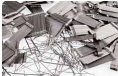
Fig. 5-3: Steel fibers for improving energy absorption of concrete
