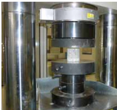
Fig. 8-15 / 16: Core drilling from sprayed concrete sample (left) and compressive strength measurement of a drill core (right)
