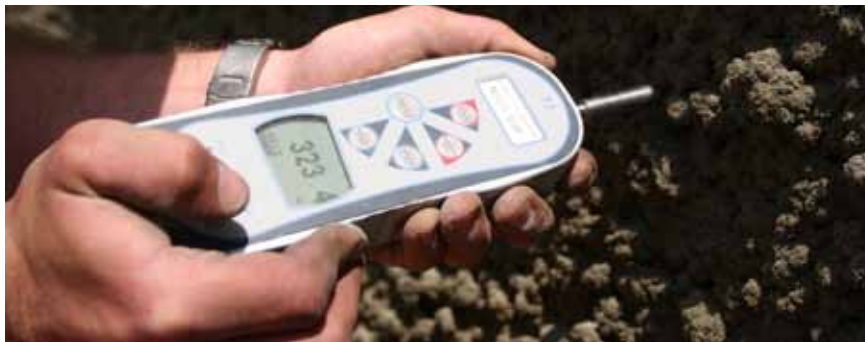
Fig. 8-12: Penetration of freshly sprayed concrete using a digital penetrometer (Mecmesin AFG 1000)
