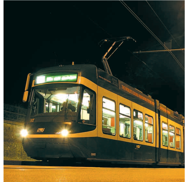
Fig. 1: Modern trams owe their stylish looks to a combination of glass, plastics and lightweight metals, bonded together with adhesives.
