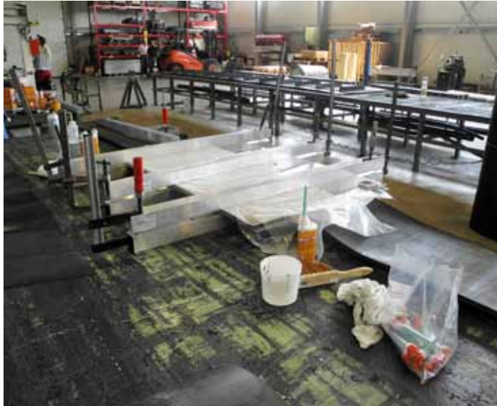
Bonding of conveyor belts in the workshop.
