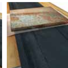
Add some pressure using a steel or a wood plate
