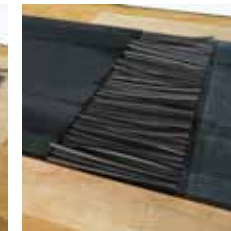
Place a plate of vulcanized rubber beneath the steel cords
