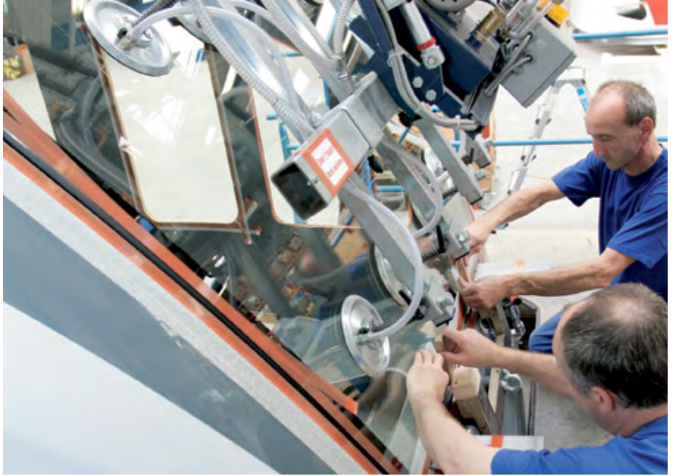
The windscreen is fitted
