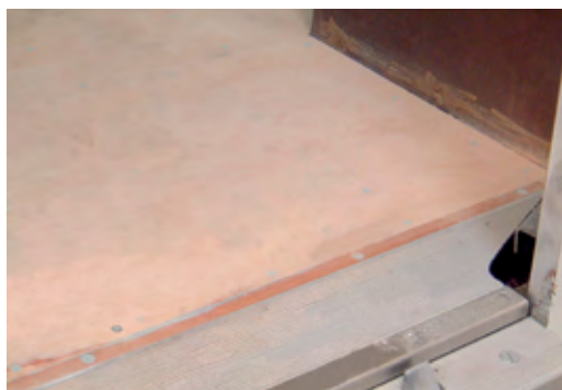
Plywood flooring is cut to size and bonded to the chassis using Sikaflex® Plus Booster. The floor is finished with a floorcovering bonded with SikaSense®.
