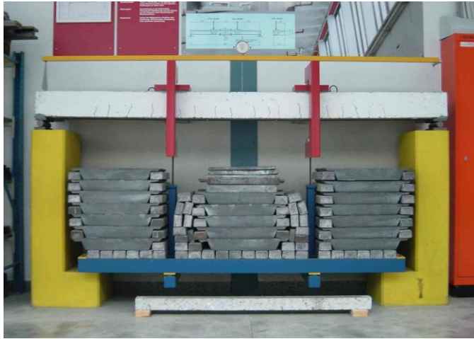
1970 Long Term Test at EMPA Sikadur® -30 (not finished yet)
